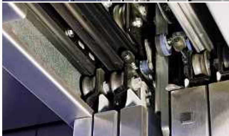
Smooth door operation guaranteed: The long life guide rollers
